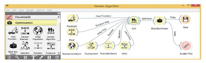
Figure 1: GA scheme assemblage using the visual Goldenberry-GA software components.
