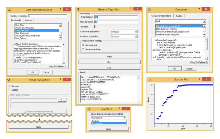
Figure 2: User interfaces for some of the Goldenberry-GA components in Figure 1. Clock-wise from bottom left: InitialPopulation, CostFunctionBuilder, GeneticAlgorithm, Crossover, ScatterPlot, Selection.
